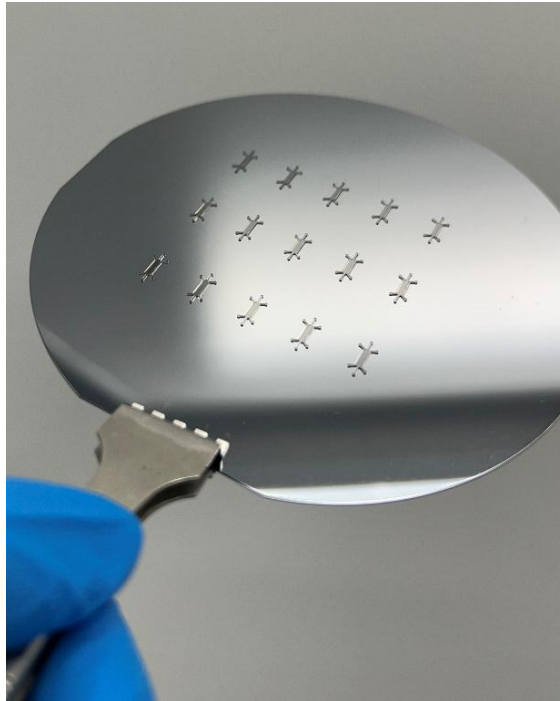
Figure 20 - Mold Version 1 fabricated on wafer substrate.
