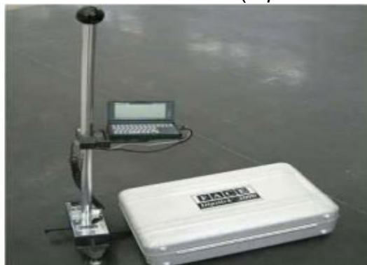
Figura 16 - Leitor de F-Numbers ( Dipstick Floor Profiler )
