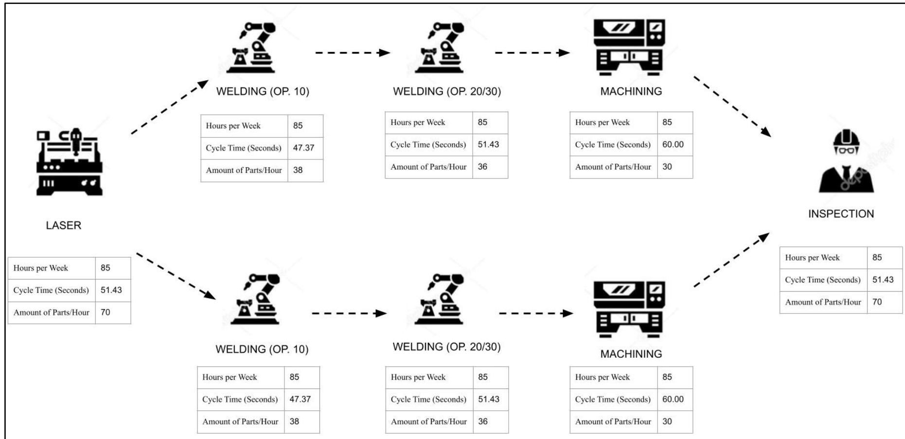
Figure 7 - Operations and production process
