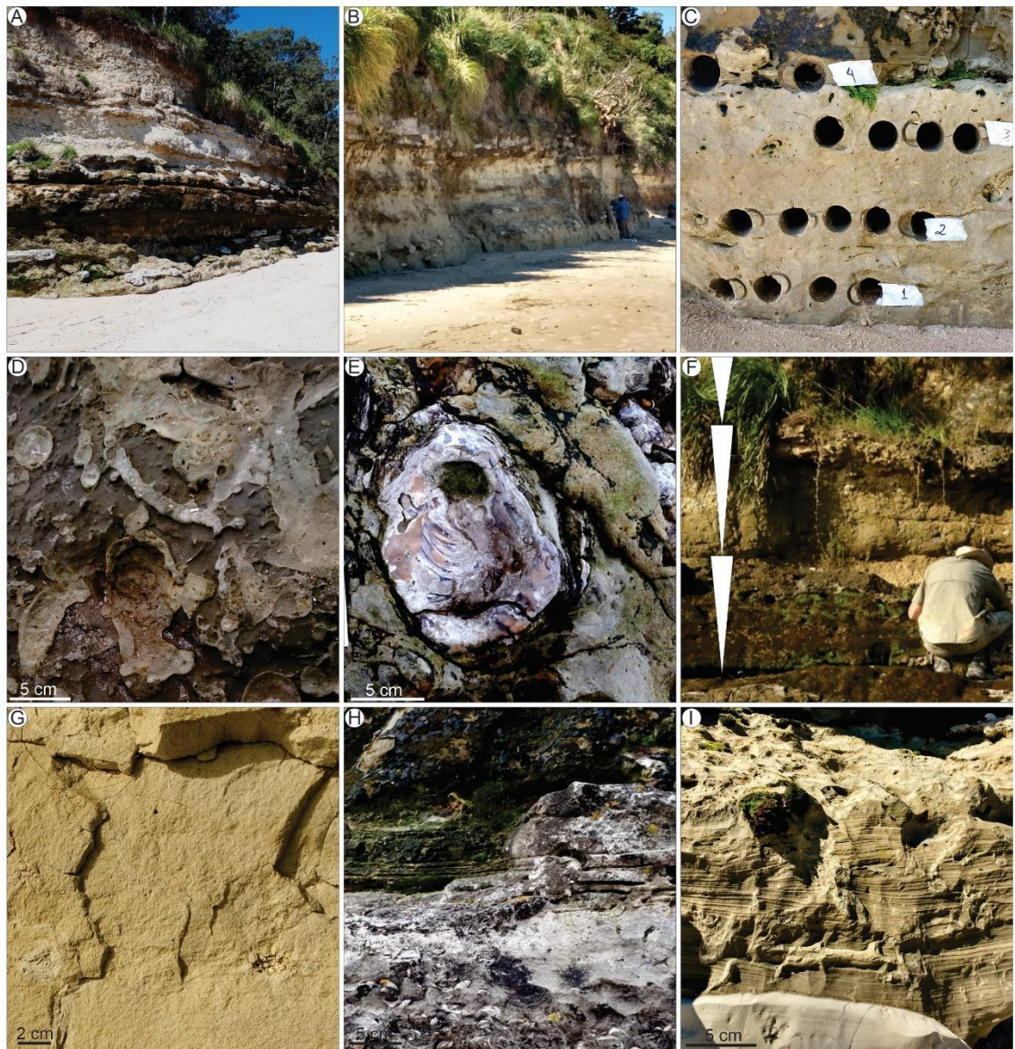
Figure 2. Sedimentary facies from Camacho Formation. A – General view of the San Pedro outcrop (FC01); B - General view of the El Chileno outcrop (FC02); C – Detail of regularly spaced collected samples; D – E. Detail of highly-bioturbated sandy siltstone (D) interbedded with an oyster bank (E). F – Cycles of fine-grained heterolithic beds (very fine-grained sandstone, siltstone, and claystone) capped by fine-grained sandstone with wave bedding. G - Fine-grained sandstone beds at top of El Chileno outcrop. H, I – Gently lenticular sandstone beds, forming a quasi-tabular geometry (H) and hummocky cross-stratification (I).
