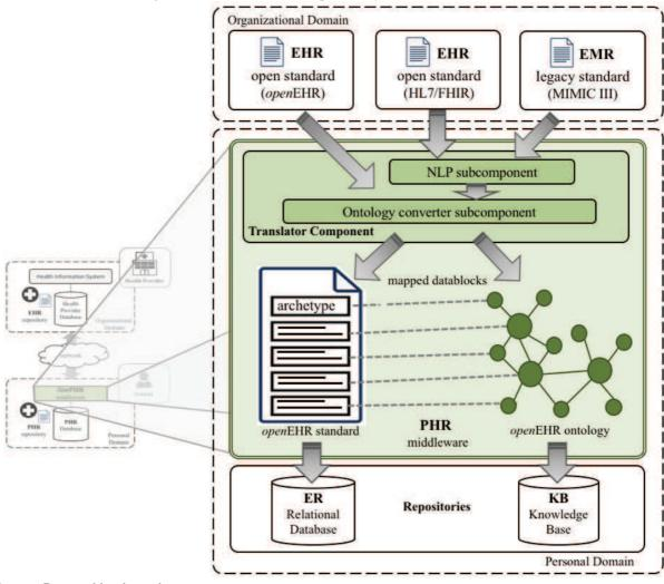
Figure 15 – Semantic interoperability detailed architecture.
