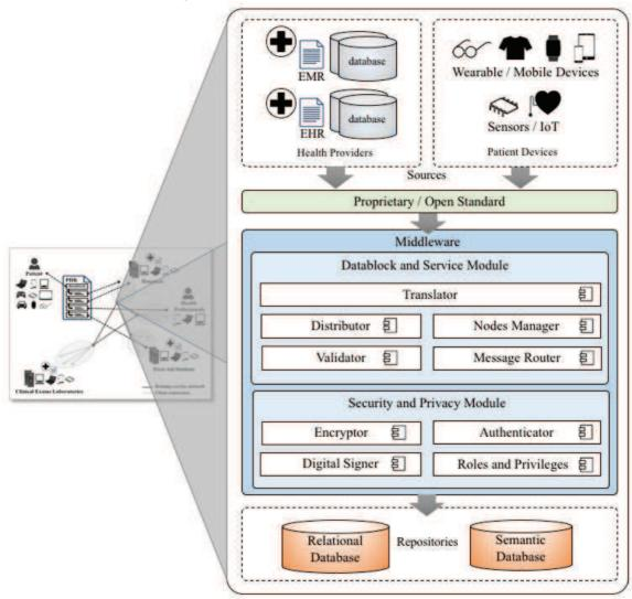
Figure 8 – OmniPHR architecture model.
