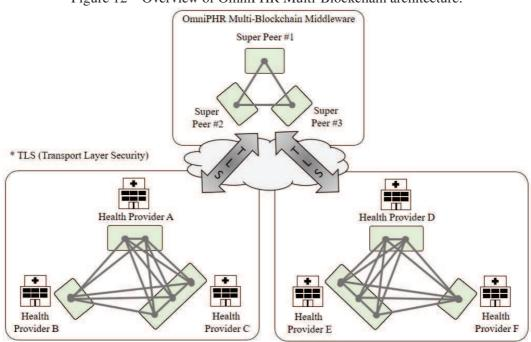
Figure 12 – Overview of OmniPHR Multi-Blockchain architecture.
