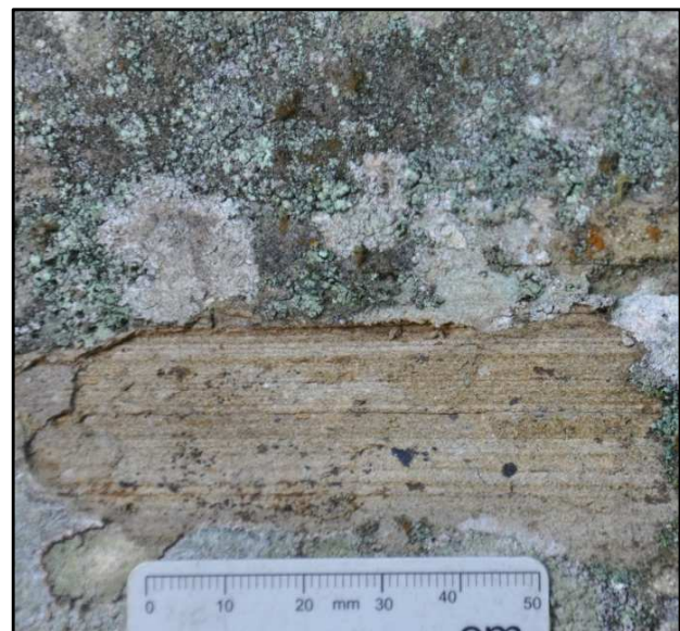
Fig. 100: Example of the laminated sandstones facies (SI). These facies appears usually at the top of graded beds.
