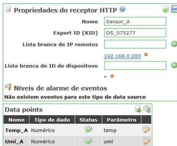
Figura 49 - Data Source receptor HTTP com respectivos Data Points
