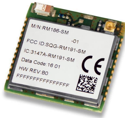
Figure 18 – Laird RM186 board.
