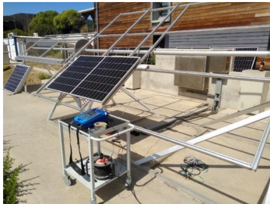
Figure 3-20: I-V tests with the bifacial modules, individually for each face
