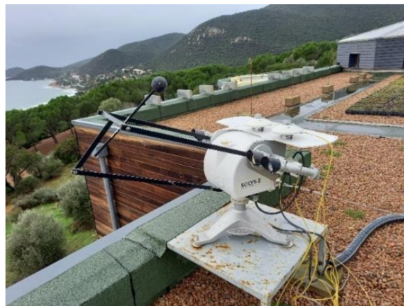
Figure 3-16: Tracker assembly to measure GHI, BNI and DHI
