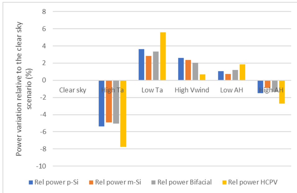
Figure 5-16: Power variations relative to the clear-sky scenario, per scenario and PV technology
