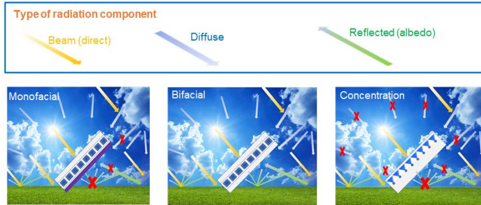
Figure 1-2: Different PV modules and usable radiation components
