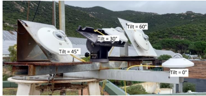
Figure 3-14: Pyranometers for tilted global irradiance measurement.
