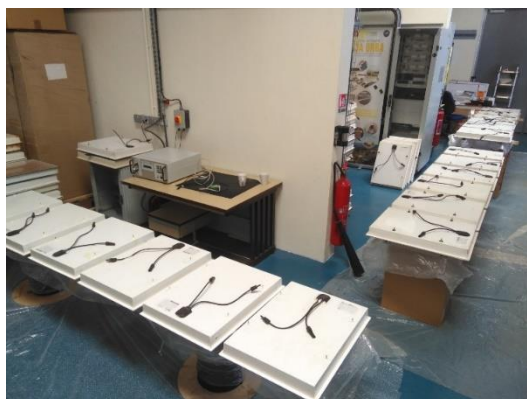
Figure 3-21: Cleaning and inspection of all HCPV modules
