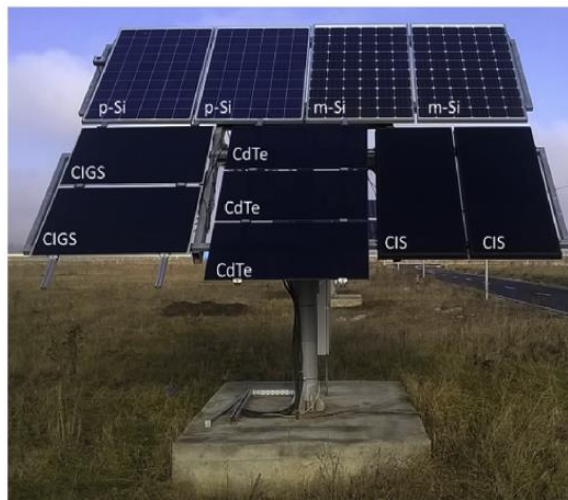
Figure 2-22: Tracking PV system assembly
