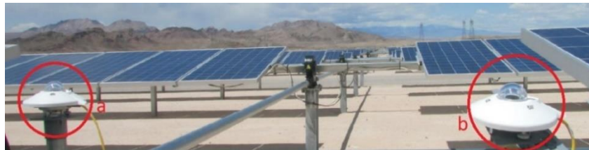
Figure 2-12: Pyranometers for monitoring GHI (a) and GNI (b)
